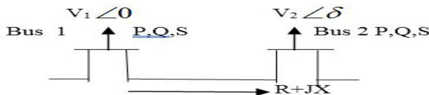
Fig3.1 Two Bus Power System Model
